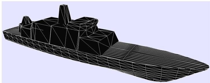
Figure 2: FAC Hamina-class triangulated model imported to CAST
