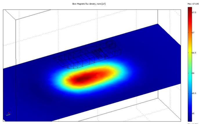
Figure 3: Magnetic signature of a simplified model
