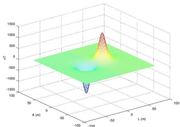
Figure 4: Magnetic signature level at a given depth
