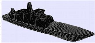
For RCS analysis SURMA currently provides only a one-way link for outputting the geometry of the vessel's outer surfaces as a triangulated surface representation in a file format accepted by an RCS calculation software CAST, which is developed and owned by the Technical Research Center of Finland and used by the Finnish Navy.
